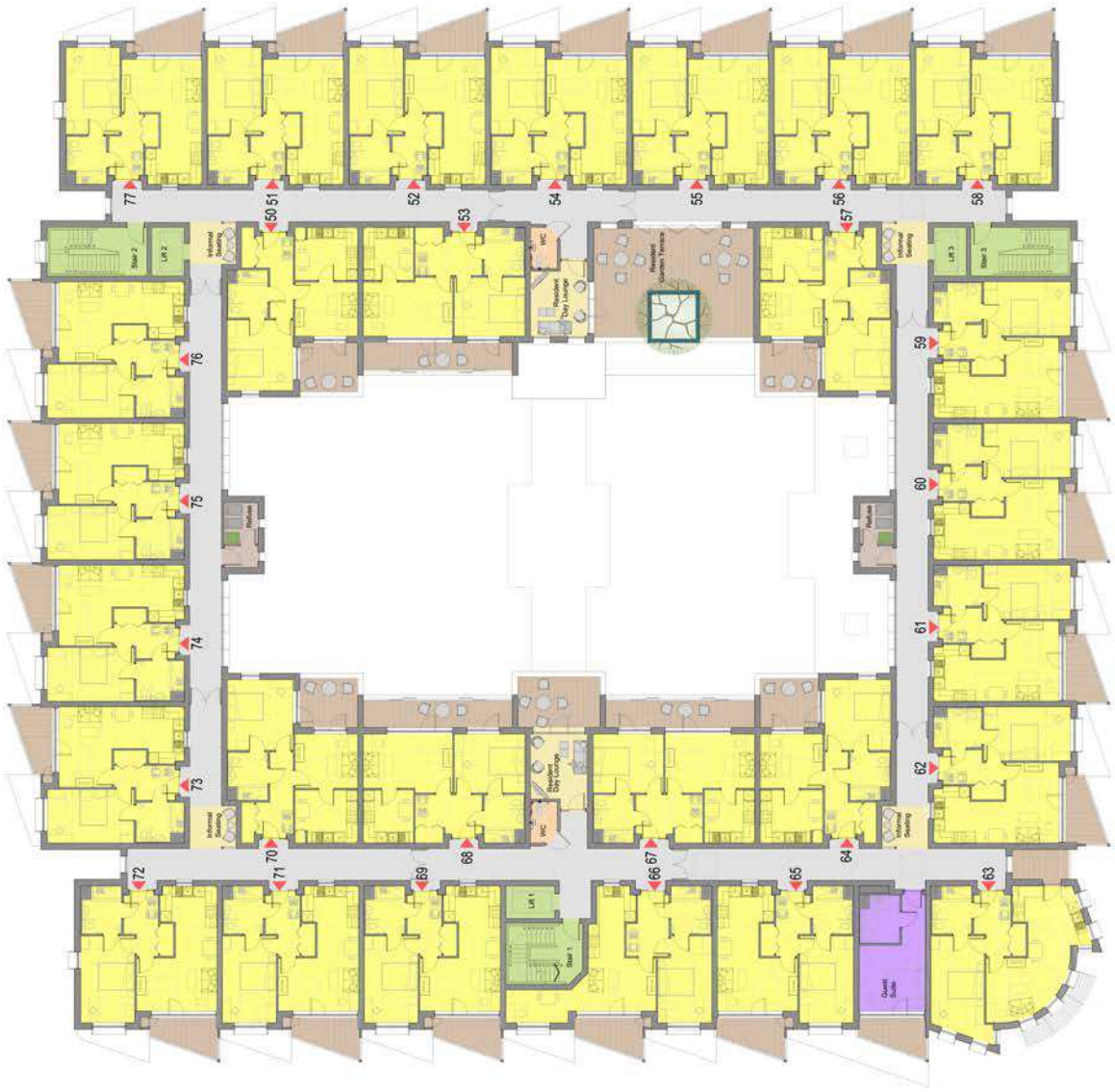
Proposed Second Floor Plan 1:100@A0 Apartments Numbers 50 to 77 (all 1-bed @ 52.5sqm)
