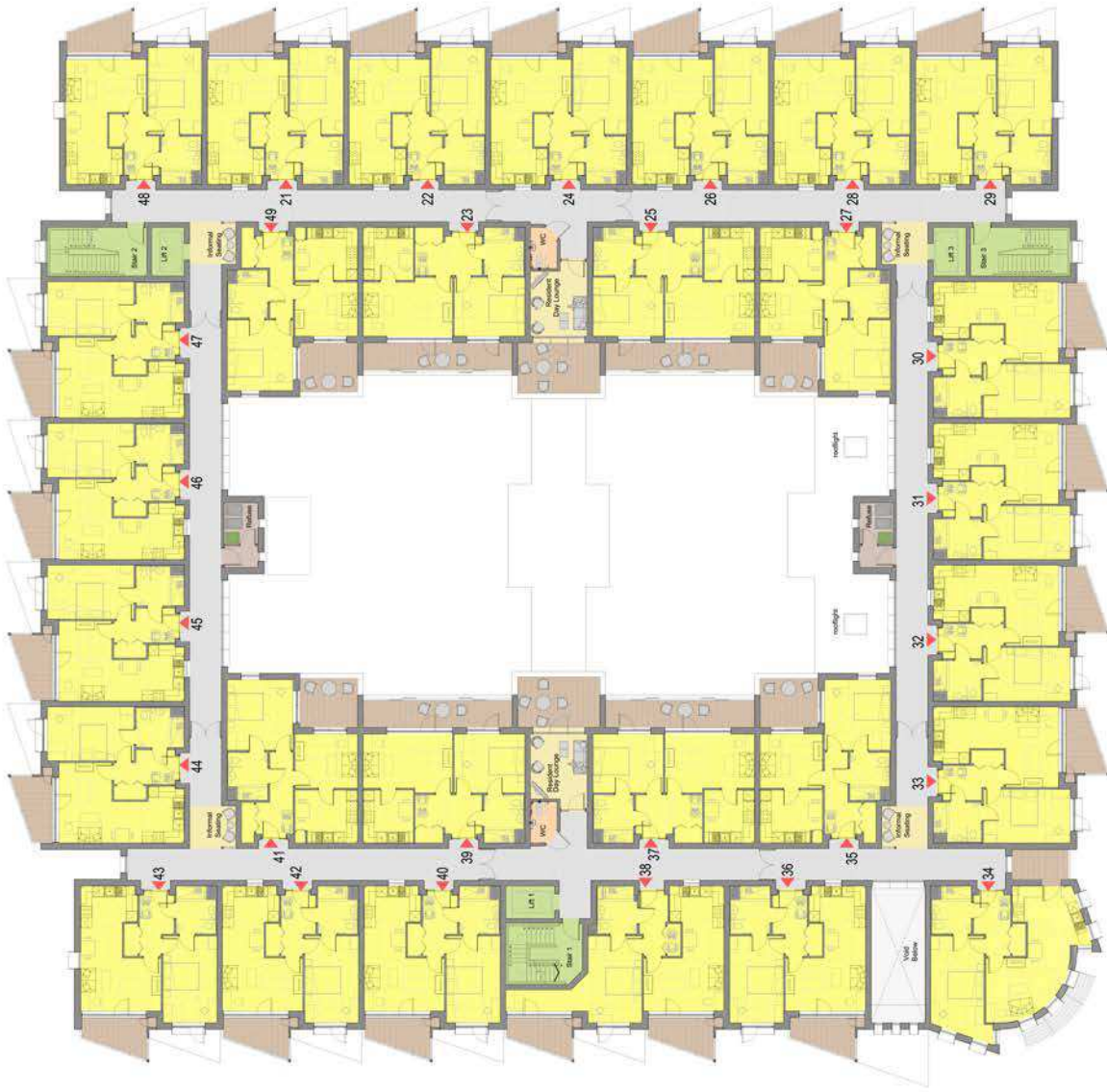
Proposed First Floor Plan 1:100@A0 Apartments Numbers 21 to 49 (all 1-bed @ 52.5sqm)
